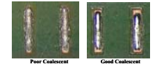
Figure 9. The excellent coalescence of NC-SMQ® 230 is evident in the above micrograph on the right.
