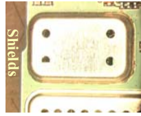
Figure 11. The shield whose joint cracks were evaluated in the drop test.
